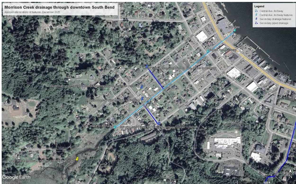
Figure F-3. Approximate Morrison Creek drainage pathways through downtown South Bend. The map identifies open-ditch reaches, primary and secondary piped drainage, the Central Avenue Archway alignment, and the outlet and tide gate at the Willapa River. Features shown are approximate as of December 2025.
